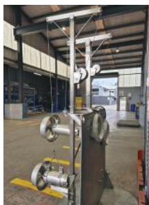
Submersible Stirrer and Lifting frame on Sump application.
